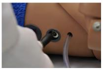
2. Connect the communication cable to the wired communication port
