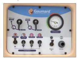
To operate the simulator, first pressurize the system using the manual air pump included. Then, activate and deactivate features using the control panel to simulate complications as the student provides care.
